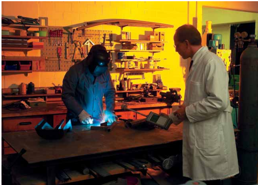
Arc welding also generates electromagnetic fields, which can represent a risk to health.
