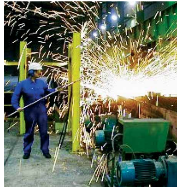
Noise measurements at a hot saw in a rolling mill to work out a noise register.
