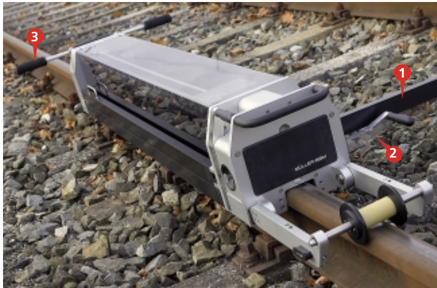
Instrument on rail, right outrigger extended (1), clamping lever activated (2), handles folded out (3)
