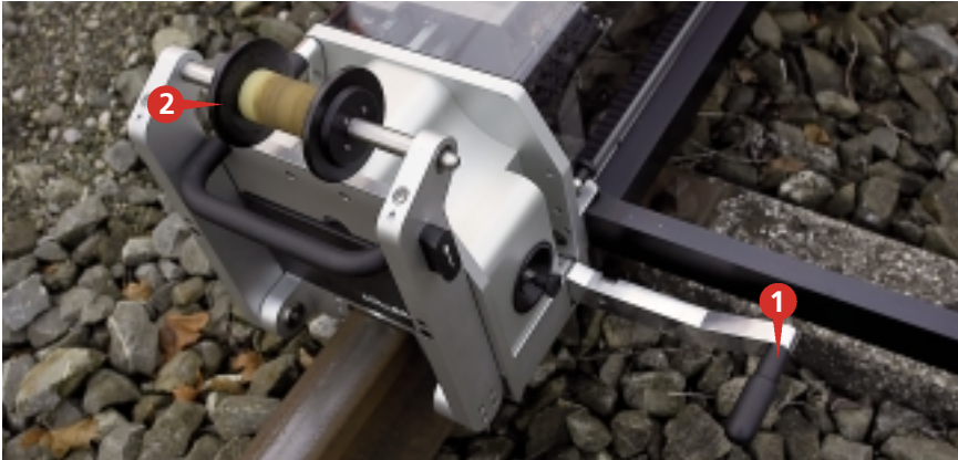
Battery compartment side: Clamping lever (1), tail wheel lifted (2)
