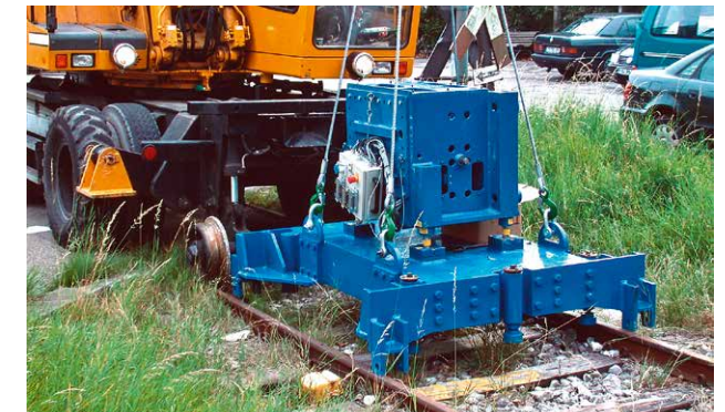
Installation of DYNAQ® on a rail track
