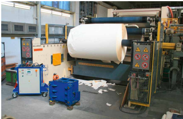
Dynamic excitation of the base frame of a paper machine
