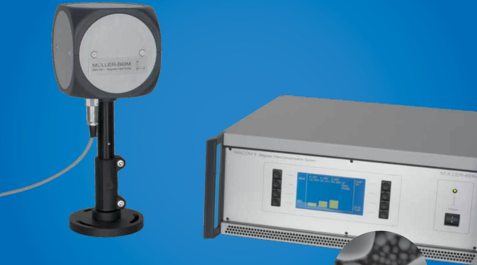
High-precision system to reduce interfering magnetic fields
