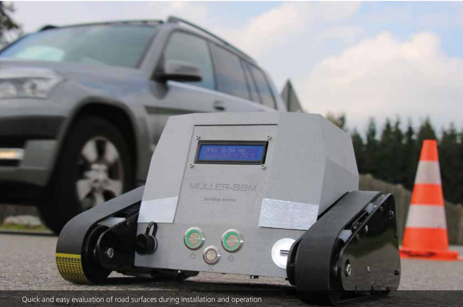
Quick and easy evaluation of road surfaces during installation and operation
