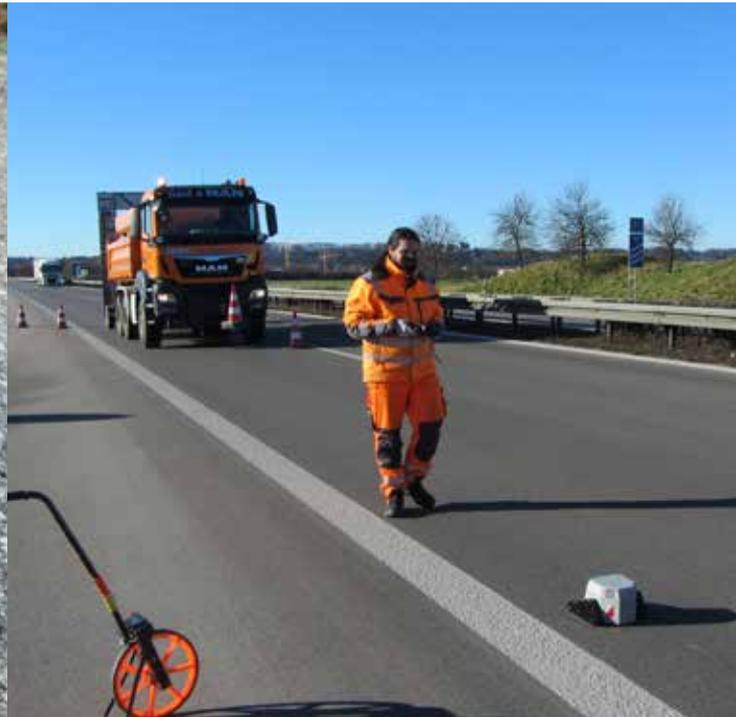
**surface drone** is a portable, light-weight and self-propelled measuring system that delivers texture data in real-time even for long measurement sections.
